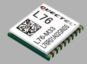
L76 series, the smallest GNSS module, is concurrent GNSS receivers and can receive and track multiple GNSS systems. With 33 tracking channels, 99 acquisition channels, and 210 PRN channels, L76 series can acquire and track any mix of GNSS signals. L76 series module contains 3 variants: L76(GPS+GLONASS), L76B(GPS+BeiDou) and L76G(GPS+GLONASS+Galileo)\*, which provides enough combination of GNSS to meet the demands of different areas.
